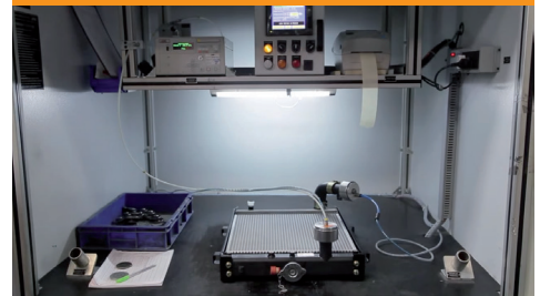
Leak / Pressure test >
