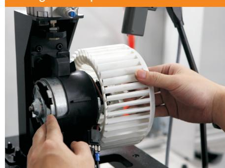
Most common reasons for interior blower failure are failures in the vehicle's electrical system, reduced flow in the air intake system and improper product handling during installation.
