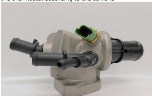
Compared with the conventional thermostat, the MAP thermostat can be open at a predetermined time through a heating cartridge and determine the degree of opening of the thermostat according to the current engine load condition, which can ensure that the engine is maintained at an optimal working temperature.
