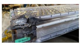
High temperatures can accelerate the degradation processes of electrode materials and electrolytes, leading to a reduction in battery capacity and life.
