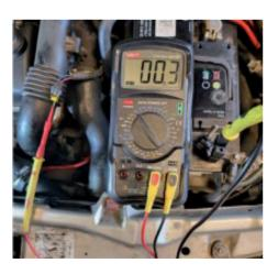
In the case of no connection, check the continuity of the red-white wire between points: pin no. 45 (of the ECU's B connector) and pin A of the sensor's plug. The engine control unit is located above the valve cover on the rear. Following the marks on the ECU's socket, locate pin 45. If the wire is broken, locate the damage and repair the wiring harness according to the manufacturer's technology.
