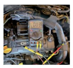
7. Measure Point A for connection to ground - the multimeter should show connection (ignition switch off).
