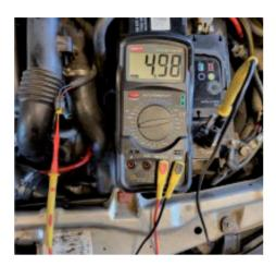
In the case of a lack of voltage, check the continuity of the power wire between points: No. 42 (of the ECU's B connector) and pin B of the sensor plug. For this purpose, remove plug B from the ECU (ignition off). The engine control unit is located, above the valve cover on the rear. Following the marks on the ECU's socket, locate pin no. 42. If the wire is broken, locate the damage and repair the wiring harness according to the manufacturer's technology.
