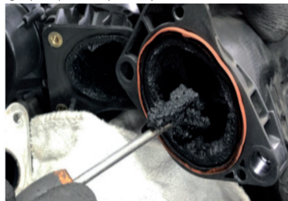
fig. 3 System permeability limited by excessive carbon contamination
