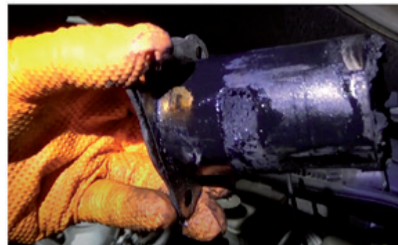
fig. 2 Original EGR valve removed from the vehicle
