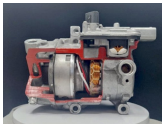
Pic 1 Cutted electrical compressor NRF
